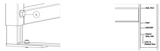
Open the 4 screws on the bottom bracket (A) and adjust the height according to toilet type (use a level). Tighten the screws at the correct height. Refer to the Label located on the upper right hand corner of the mounting frame for the correct height.
