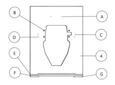
Using the 4 fastening holes (A) ( $\emptyset$ 8.5), secure the frame to the wall. See extra mounting support for additional fastening.
