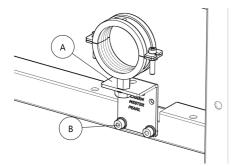
Adjust the clamp bracket according to the toilet type.
